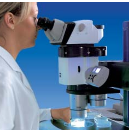
Screening of C. elegans with the SteREO Discovery.V12 equipped with the PentaFluar S module and the X-Cite 120 Fl illuminator.
