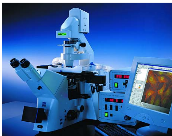
Figure 1 Cell Observer: the Axiovert 200 mot microscope with climate box, Axiocam HR digital camera, and Axiovision image processing system.
