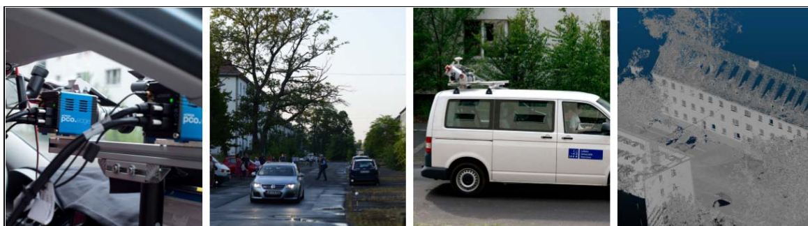
Figure 1. Dataset acquisition. Reference Data (in this case stereo) generated using auxiliary modalities such as LIDAR (right two panels) are subject to measurement uncertainty. [1]
