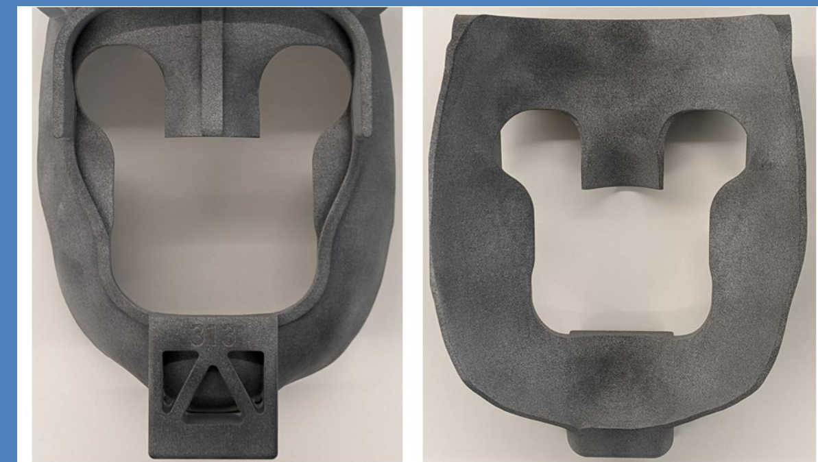
Figure 1 – An example of front (left image) and back (right image) of 3D printed personalized patient interface for self-alignment of patient with imaging device.
