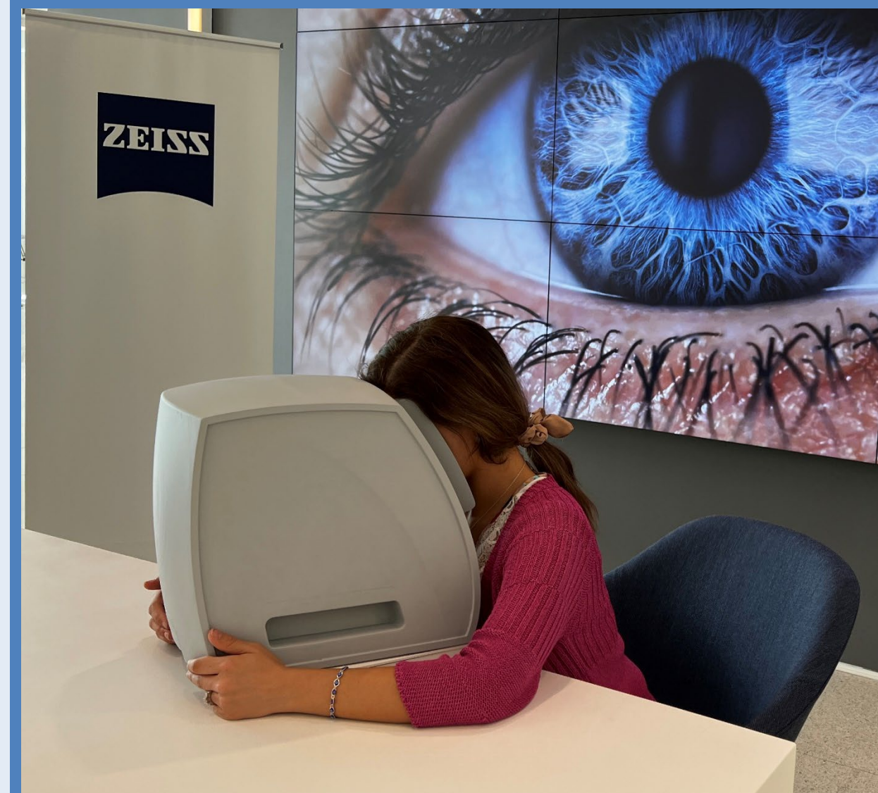
Figure 2 – Patient using low-cost OCT prototype system with self-triggered acquisition and personalized patient interface developed at ZEISS, Dublin, CA.
