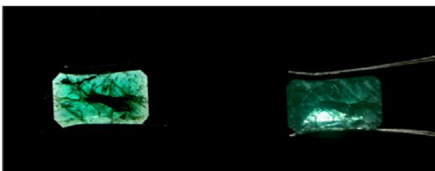
**Figure 7** Synthetic emerald (Chatham), observed with and without an immersion medium in polarized transmitted light. Using an immersion medium with a refractive index similar to that of the precious stone minimizes surface reflections and makes the internal structure of the stone visible.
