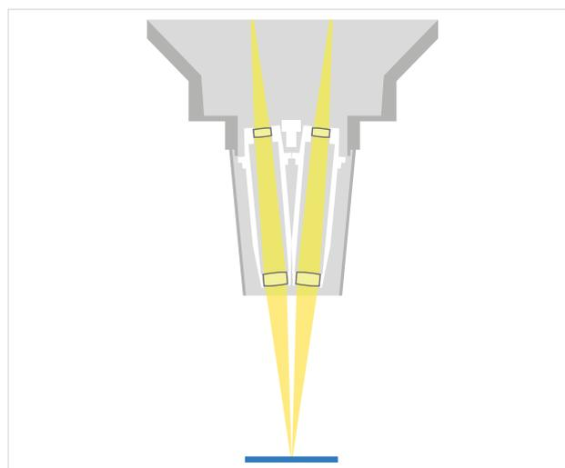
**Figure 1** Beam path of a Greenough-type stereo microscope
