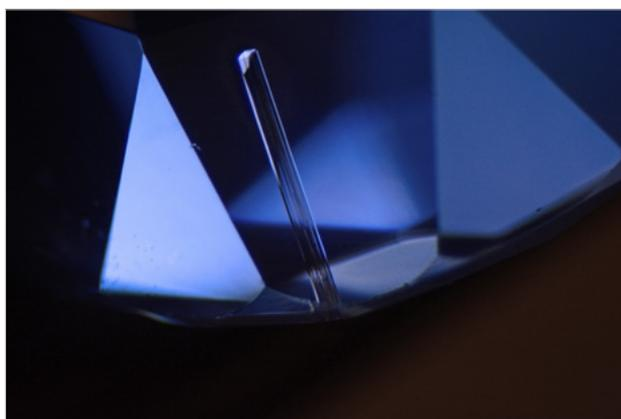
**Figure 4** Prismatic green hornblende inclusion (amphibole) in sapphire from Kashmir, India. The inclusion was identified using Raman microspectroscopy. These types of green hornblende needles are a characteristic inclusion in sapphire from India and allow experienced gemologists to determine the origin of the cut sapphire in a piece of jewelry. GEMMASTER with ZEISS Stemi 508; dark-field illumination, magnification: 50x
