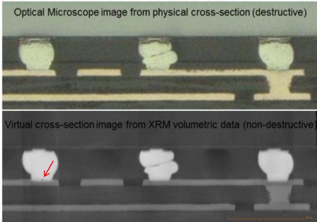
**Figure 1:** Comparison between images collected with an optical microscope taken after destructive cross-sectioning (top) and a virtual cross-section image taken from the non-destructive XRM scan (bottom).
