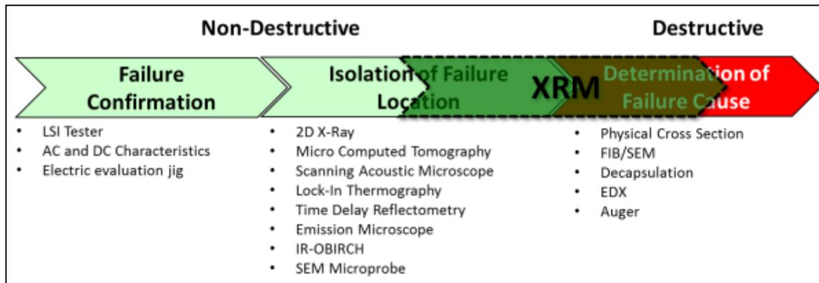
**Figure 3:** Proposed use of X-Ray Microscopy (XRM) to replace mechanical cross-sections to streamline the Failure Analysis Workflow and shorten the time-to-market of 3DIC process development.
