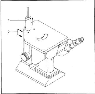
Connect microscope to line supply; knob (1.11) must be switched off. Then switch on halogen lamp with this knob. Swing an objective into light path.
