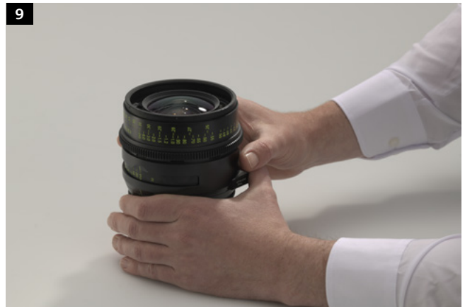
Put the ring back on the lens. The desired scale unit is now visible in the window of the scale reading.
