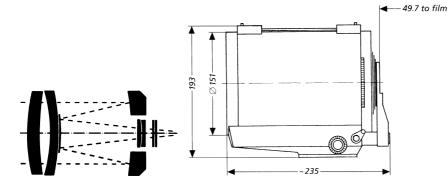
The basic design of the **Mirotar**<sup>®</sup> - concave primary mirror with a hole in the center and convex secondary mirror - is similar to the design frequently applied in astronomical telescopes. It further contains two lens elements in front of and two behind the mirror surfaces. They reduce the aberrations caused by the mirror to a minimum.
