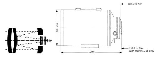
The basic design of the **Mirotar**<sup>®</sup> lens - concave primary mirror with a hole in the center and convex secondary mirror - is similar to the design frequently applied in astronomical telescopes. It further contains two lens elements in front of and two behind the mirror surfaces. They reduce the aberrations caused by the mirror to a minimum.
