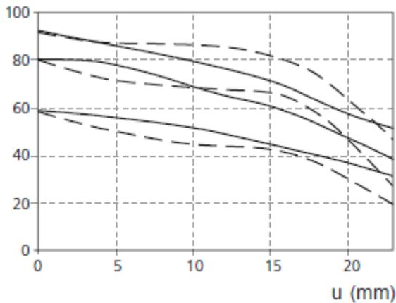
The Modulation Transfer (MTF) as a function of image height (u) and slit orientation (sagittal, tangential) has been measured with white light at spatial frequencies of  $R = 10, 20$  and  $40$  cycles/mm. The MTF charts are valid for the ZM-version and for white light.
