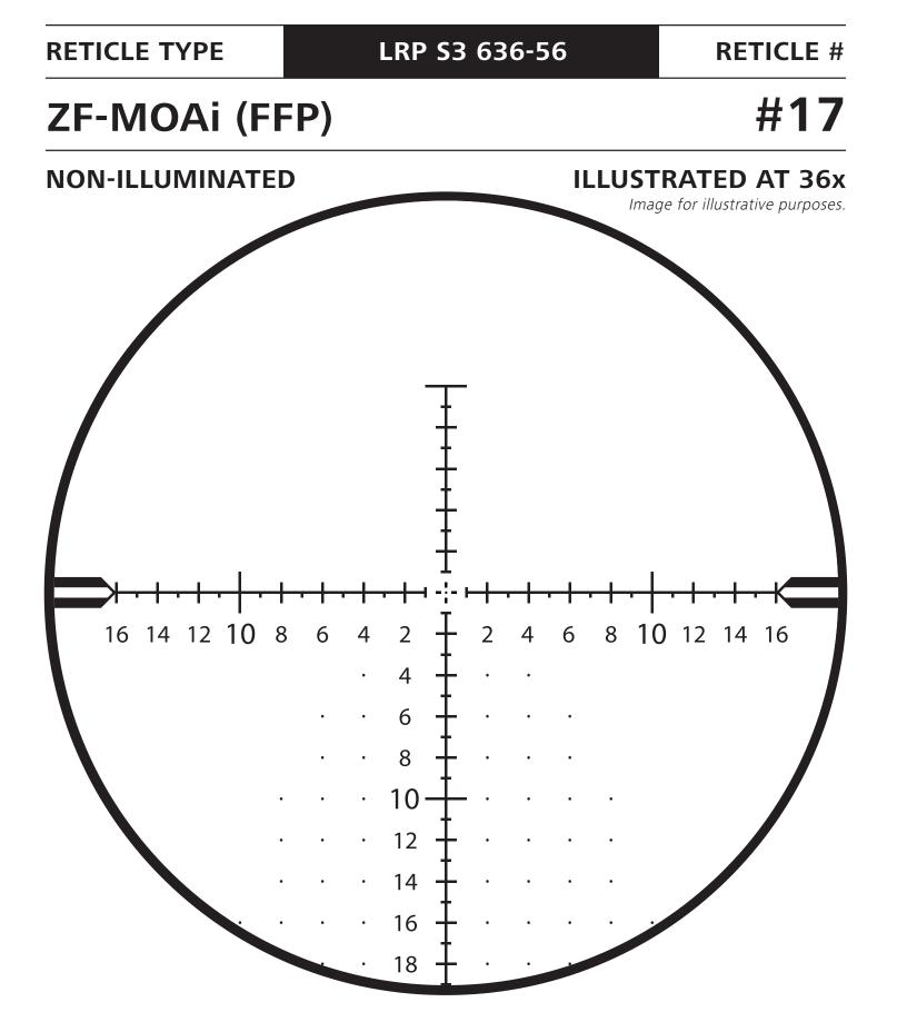
ZF-MOAi = ZEISS First Focal Plane - Minute of Angle, illuminated
