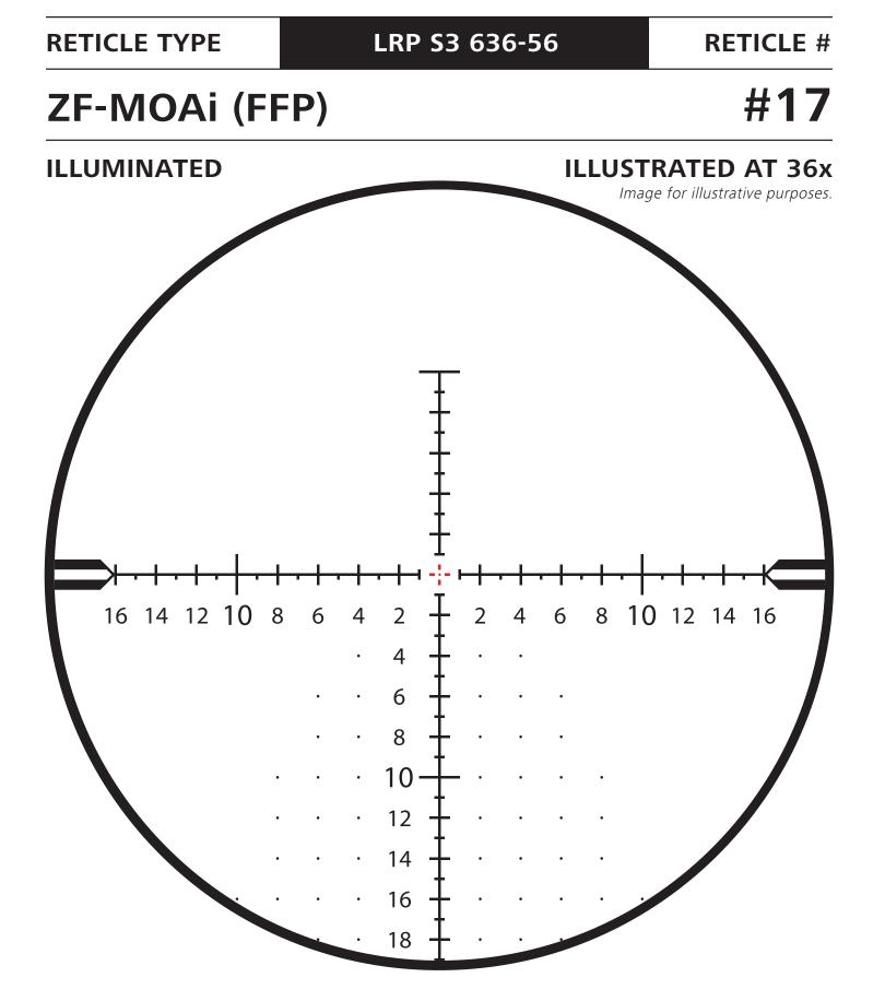
ZF-MOAi = ZEISS First Focal Plane – Minute of Angle, illuminated
