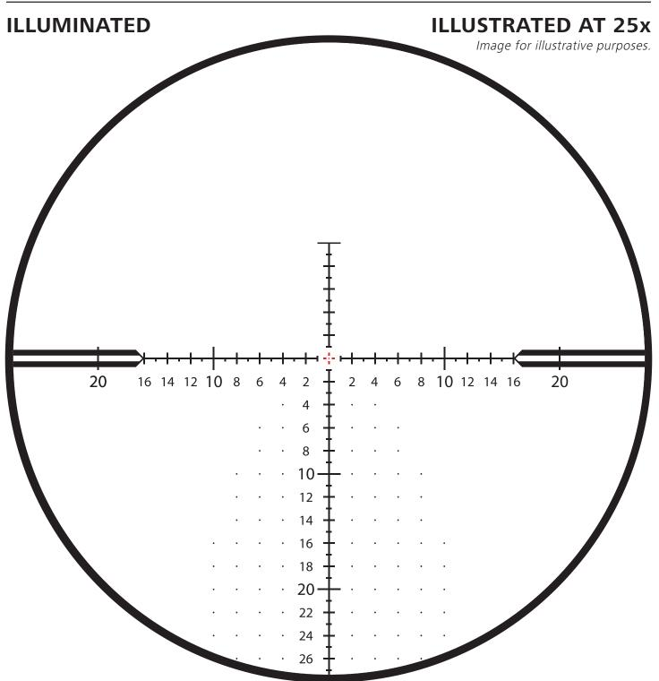
ZF-MOAi = ZEISS First Focal Plane - Minute of Angle, illuminated
