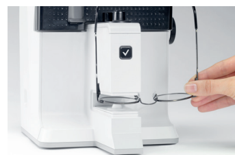
Measurement of UV transmission.
