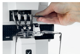
Easy to refill marking system with 3 marking pens.
