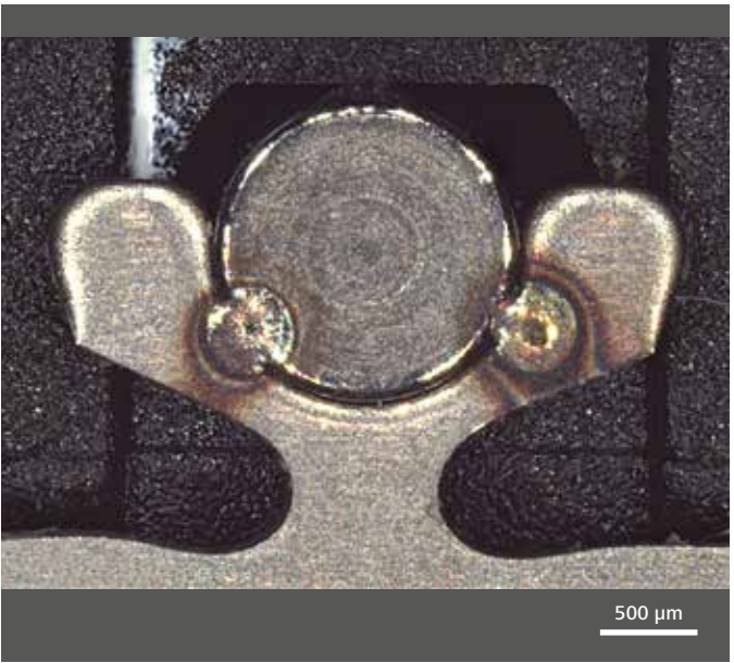
Laser welds Objective: 1.6×, expanded depth of field, LED ring illumination
