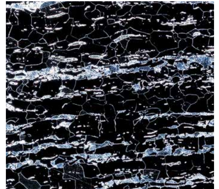
Steel structure, darkfield, objective: EC-EPIPLAN 20x/0.4
