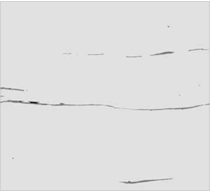
Non-metallic inclusions in steel Microscope: ZEISS Axio Imager.Z2m Objective: EC Epiplan-NEOFLUAR 10x/0.25 Camera: ZEISS AxioCam MRC
