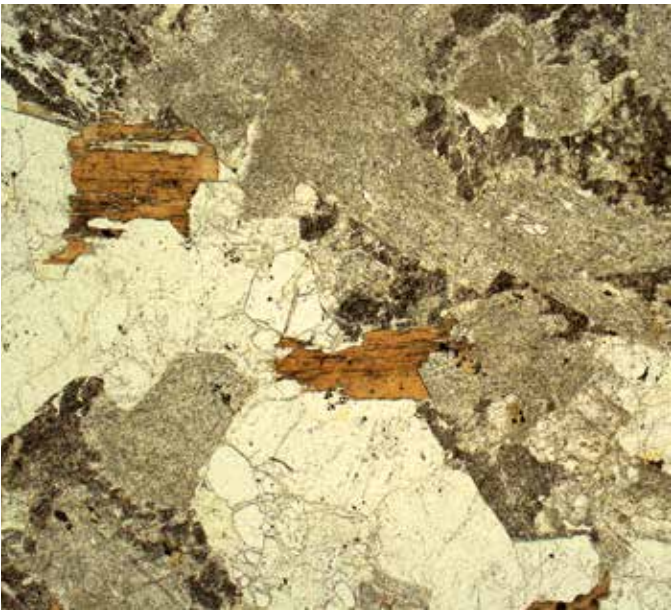
Biotite in granite; pleochroism made visible by rotating the stage; brightfield
