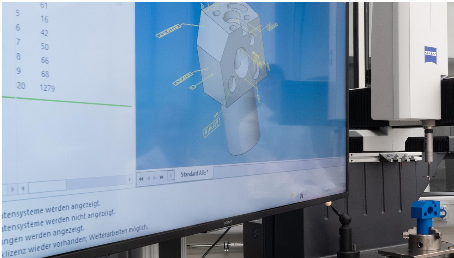
ces, and other notes are often defined separately. A drawing is derived based on the 3D geometry, in which dimensions and geometric tolerance specifications are then stored. These dimensions and tolerances become the nominal values for the measurement and are linked to a measuring point in ZEISS CALYPSO.
