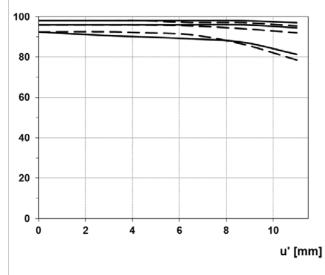
The Modulation Transfer (MTF) as a function of image height (u) and slit orientation (sagittal, tangential) has been measured with white light at spatial frequencies of R = 10, 20 and 40 cycles/mm.
