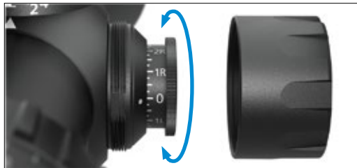
1b. Exposed windage turret. Rotate clockwise to move bullet impact left on target. Rotate counterclockwise to move bullet impact right on target.
