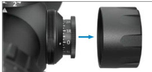
1c. Similar to the capped elevation turret, pull out the windage turret's outer ring and freely rotate it to index the zero position. Release the turret's outer ring.
