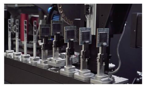
ZEISS Autoloader option enables you to program up to 70 samples at a time to run sequentially.
