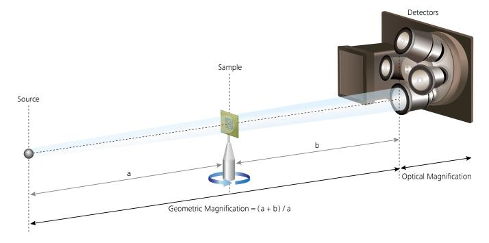
Xradia Versa scintillator-coupled optical detectors enable high resolution and contrast at long working distances.
