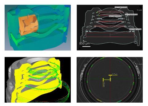
High-resolution tomography images and measurement workflow developed by Xradia Versa X-ray microscopy.
