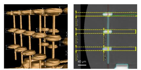
Xradia Versa RepScan results show bond line thickness measurements through stacked dies for a HBM device. 3D and a virtual slice at 0.7  $\mu$ m/voxel are shown on the left and right, respectively.
