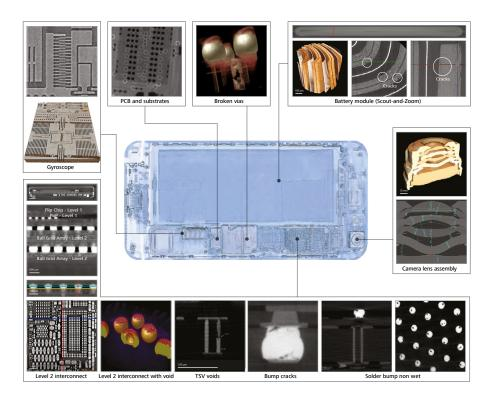
Versa XRM 3D images and virtual cross sections of defects deeply buried in a smartphones.
