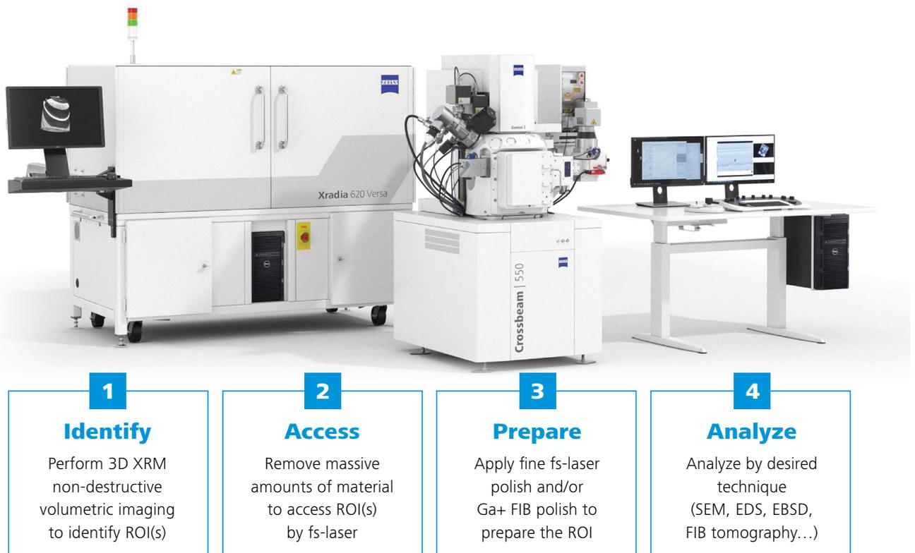
**Figure 1** Summary of the four main steps of the Cut2ROI workflow used in this study. Step 1 is performed using ZEISS Versa 3D X-ray microscopy, and Steps 2 through 4 are performed using ZEISS Crossbeam laser FIB-SEM.
