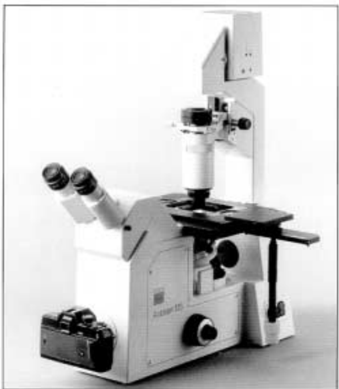
Axiomvert 135 equipped for higher illuminating aperture
