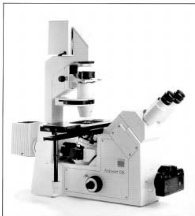
Axiomvert 135 equipped for incident-light fluorescence
