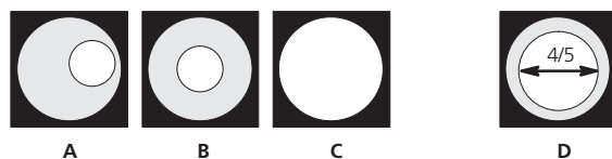
Fig. 53 Microscope setting for incident light brightfield
