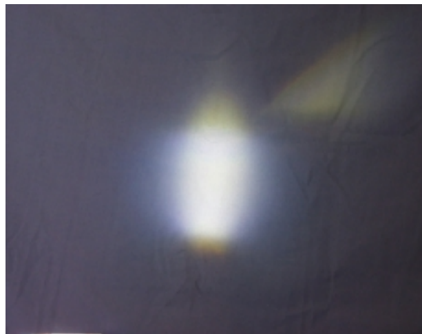
Fig. 2-23 Focal spots of HBO 103 before coarse adjustment
