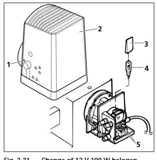
Fig. 2-31 Change of 12 V 100 W halogen lamp
