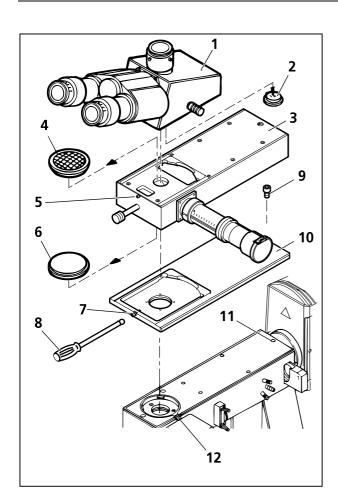
Fig. 2-7 Attachment of intermediate tube for image projection
