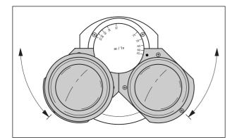
Fig. 2-12 Setting of eyepiece distance and viewing height of the binocular tube
