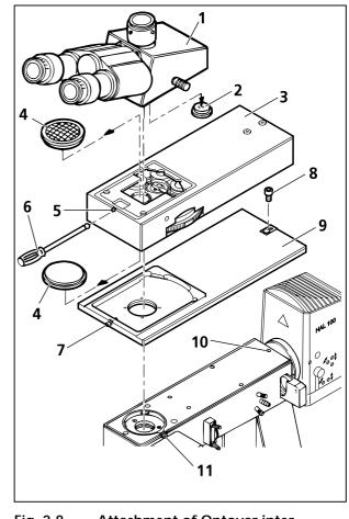
Fig. 2-8 Attachment of Optovar intermediate tube
