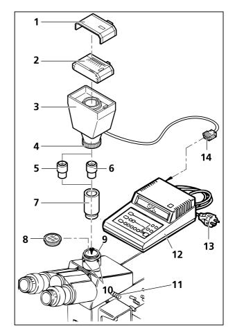
Fig. 3-30 Attachment of MC 80 DX microscope camera (35 mm format)
