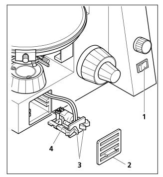
Fig. 2-32 Change of 6 V 30 W halogen lamp (Axiotech 30 and Axiotech 100)
