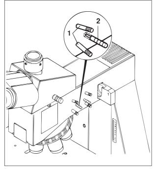
Fig. 2-22 Setting of reflected-light luminousfield diaphragm of the Axiotech 30
