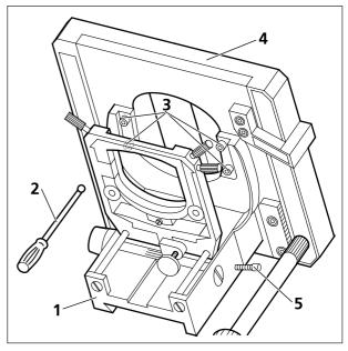
Fig. 2-16 Attachment/change of microscope stage (configuration with stage carrier D)
