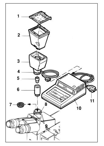
Fig. 3-31 Attachment of MC 80 DX microscope camera (large format)
