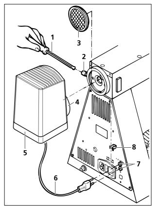
Fig. 2-29 Attachment of 12 V 100 W halogen illuminator
