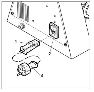
Fig. 2-24 Connecting the Axiotech 30 to the line
