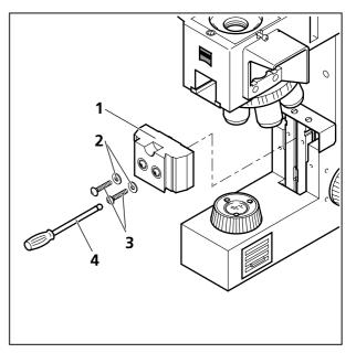
Fig. 2-15 Attachment of adapter for stage carrier D
