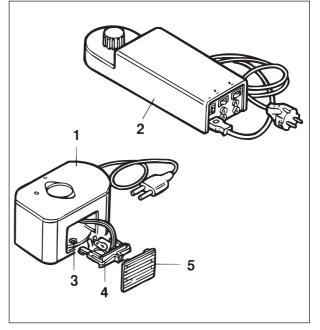
Fig. 2-34 Change of 6 V 30 W halogen lamp (Axiotech<sup>vario</sup> 100)
