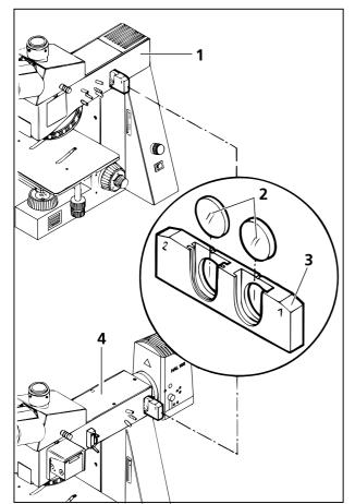
Fig. 2-20 Equip filter slider and push it in beam path
