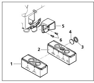
Fig. 2-21 Change of filters in reflector slider
