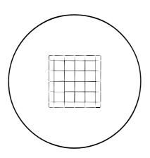
25 test points, test line length:  $25 \times 2 \times 2$  mm, test area:  $25 \times 2 \times 2$  mm
