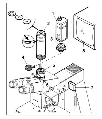
Fig. 3-32 Attachment of video camera
