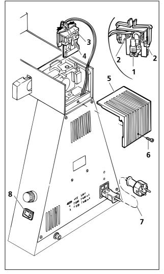
Fig. 2-28 Change of 6 V 30 W halogen lamp
