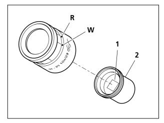
Fig. 2-11 Insertion of the eyepiece reticle
