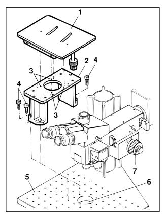
Fig. 2-17 Attachment/change of microscope stage (stage carrier H = 140 mm)
