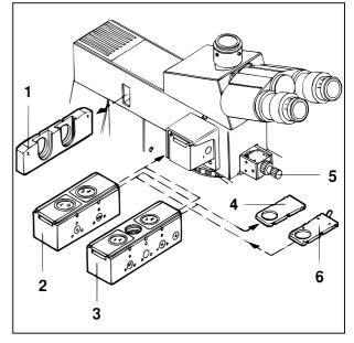
Fig. 3-14 Setting of reflected-light polarization contrast
