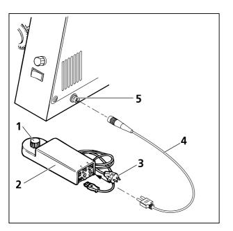
Fig. 2-33 Connecting the 6 V 30 W halogen illuminator to the line (Axiotech 30 and Axiotech 100)
