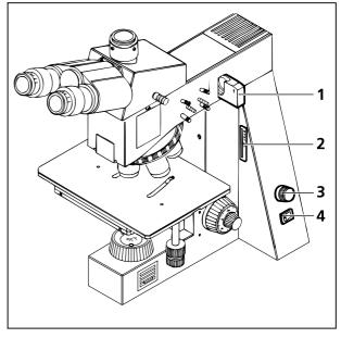
Fig. 2-25 Switching on the Axiotech 30
