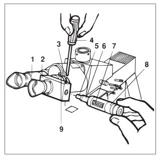
Fig. 3-35 Attachment of digital eyepiece measuring device
