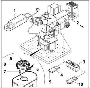
Fig. 3-24 Setting of transmitted-light polarization contrast with reflector slider HD DIC (Axiotech<sup>vario</sup> 100)
