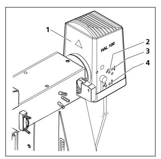
Fig. 2-30 Alignment of 12 V 100 W halogen lamp
