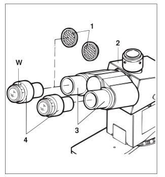
Fig. 2-9 Insertion of eyepieces
