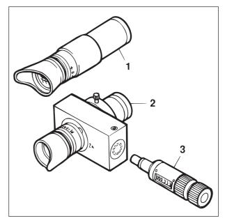
Fig. 3-34 Digital eyepiece measuring device
