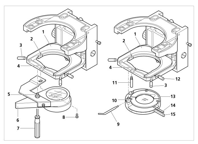
Fig. 3-23 Attach polarizer to stage carrier D
