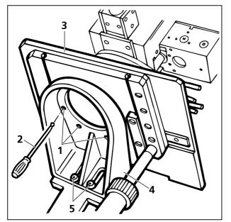
Fig. 2-14 Attachment/change of microscope stage (configuration with stage carrier A)
