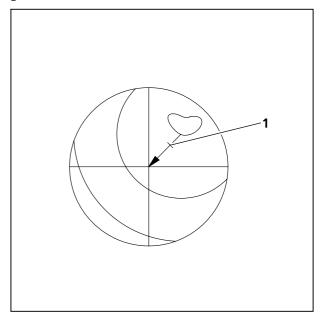
Fig. 2-19 Centering of microscope stage with maximum deflection between object detail and eyepiece reticle
