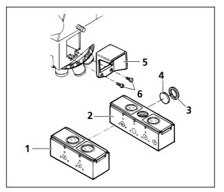
Fig. 3-19 Change of filters in the reflector slider
