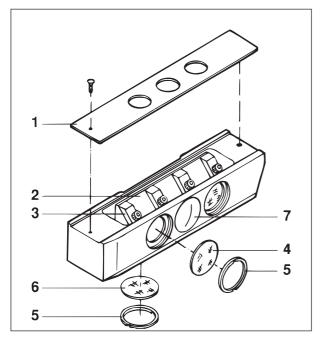
Excitation filters (3-18/4), barrier filters (3-18/6) and chromatic beam splitters (3-18/2) can be inserted and exchanged; the excitation and barrier filters are accessible and can be exchanged after unscrewing the retainer rings (3-18/5), and the chromatic beam splitter after removing the base plate (3-18/1) and loosening the mounts (3-18/3).
