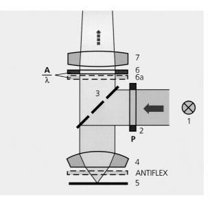
Fig. 3-13 Reflected-light polarization contrast
