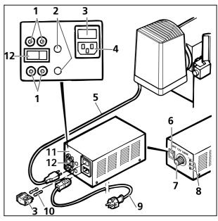
Fig. 2-27 Connecting the Axiotech<sup>vario</sup> 100 to the line via separate power unit
