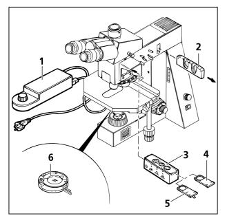
Fig. 3-22 Setting of transmitted-light polarization contrast with reflector slider HD DIC (Axiotech 30/100)
