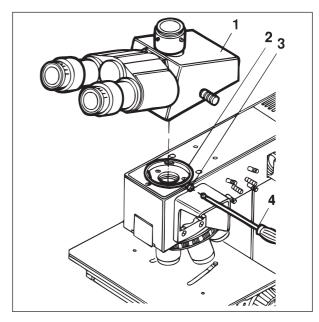
Fig. 2-6 Attachment of binocular tube
