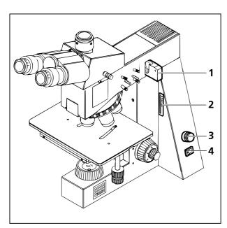
Fig. 3-4 Switch on the Axiotech 30 and Axiotech 100
