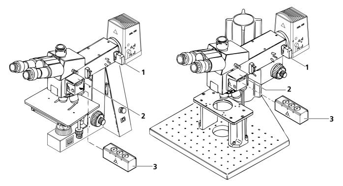
Fig. 3-17 Setting of epi-fluorescence using the 3 FL reflector slider
