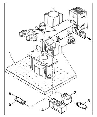
Fig. 3-26 Setting of transmitted-light polarization contrast using reflector slider without DIC position (Axiotech<sup>vario</sup> 100)
