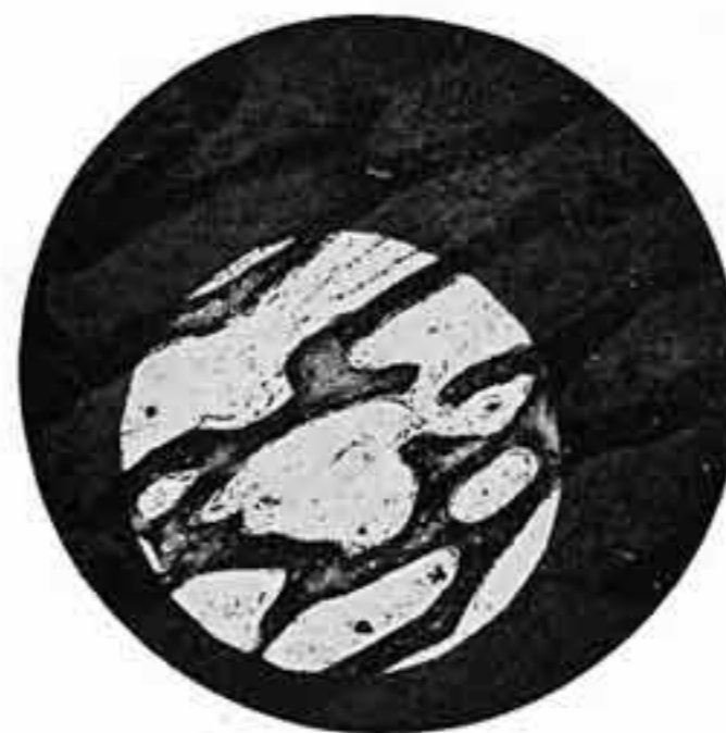
B Sharply defined luminous field stop
