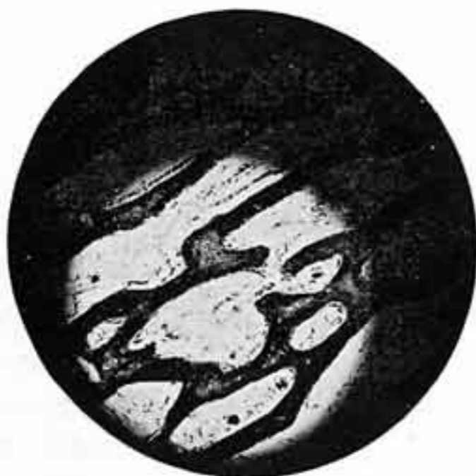
A Unsharp luminous field stop
