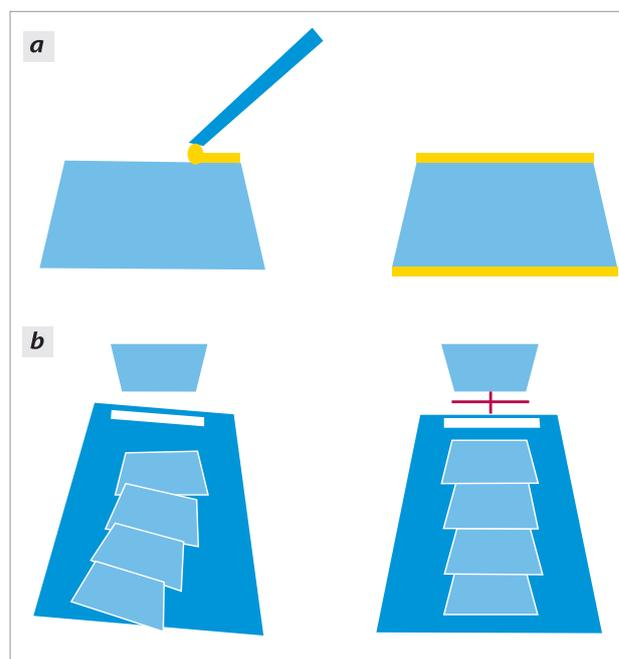
**Figure 2:** Precutting adjustments a: Superglue is placed with a tooth stick on the cutting edges to allow to produce longer ribbons. b: The right orientation of the cutting and the knife surface is essential for perfect straight orientation of the ribbons. The knife / the cutting surface have to be absolutely in parallel.
