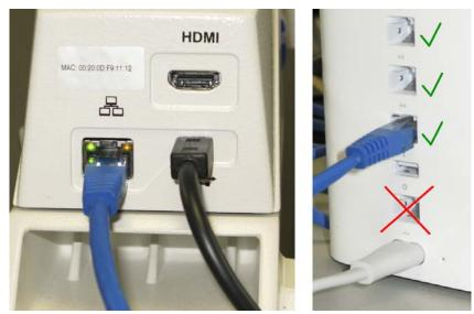
You can add up to three microscopes directly to an AirPort. If you need to connect more microscopes, consider adding an **unmanaged switch** and connecting that the microscopes to that (and the switch to the router).
