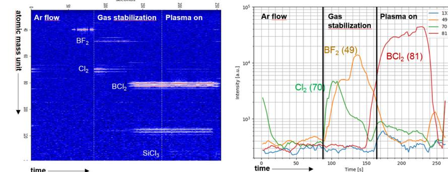
TCP/ICP etch chamber; low pressure regime (2-10 mT);  $\text{BCl}_3$  etch;  $\text{SiO}_2$  wafer
