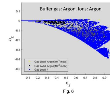
The desired cooling effect of Helium as background gas does not seem to be relevant in the given pressure regime of  $10^{-4}$  mbar. Even with argon the ion stability is not affected significantly. But this could be due to the fact, that at low pressure only few collisions between the ion and the gas load occur. Fig. 6 shows that collisions with argon at a pressure of  $10^{-2}$  mbar indeed make a huge difference for stability due to ion heating.
