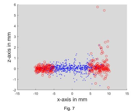
The further the ion starting positions are away from the center, the more likely they are unstable. 60% of the generated ions are effectively trapped.
