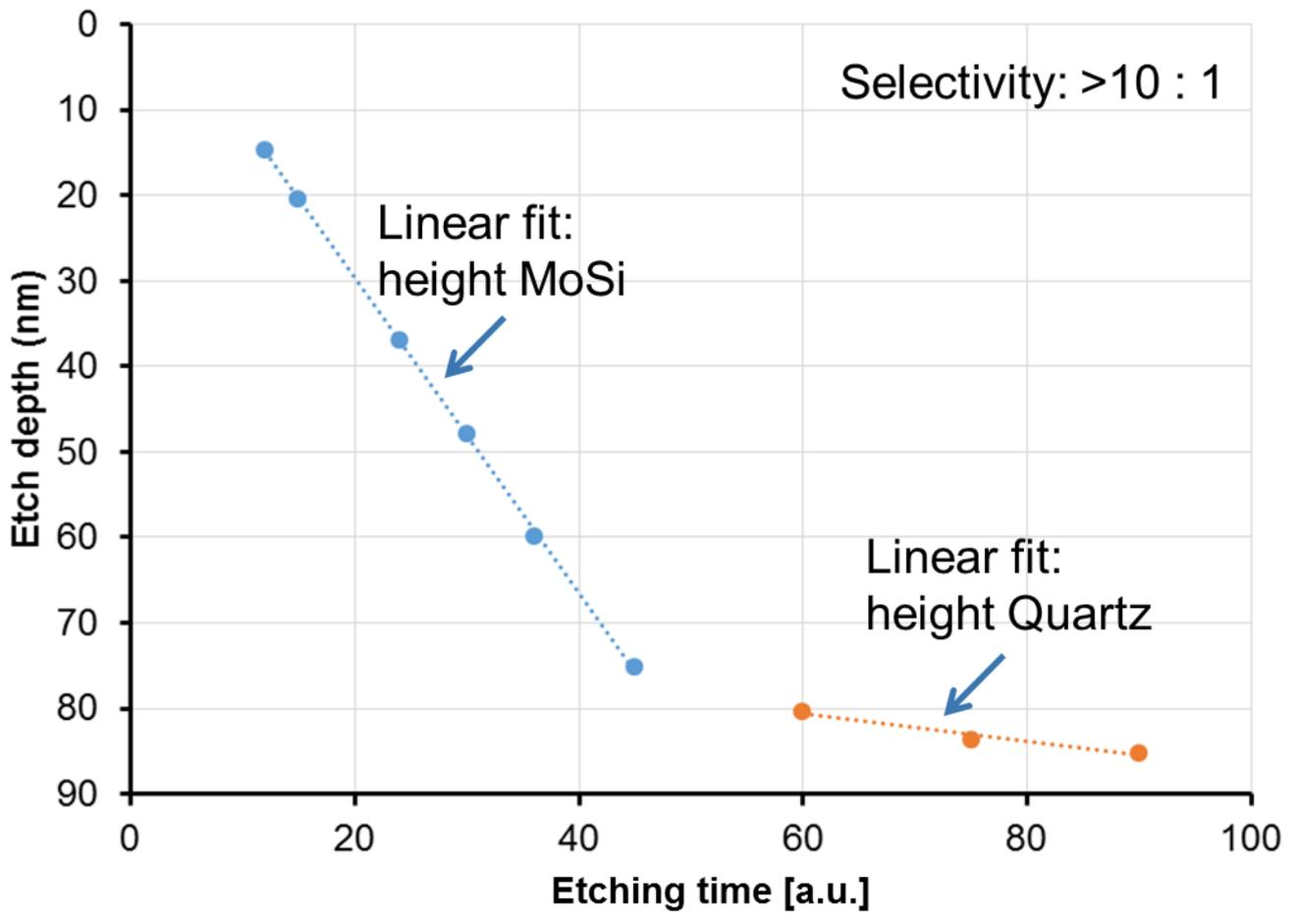
Figure 7: Selectivity data for the high durability MoSi A6L2. A selectivity between MoSi and Quartz of more than 10:1 was achieved
