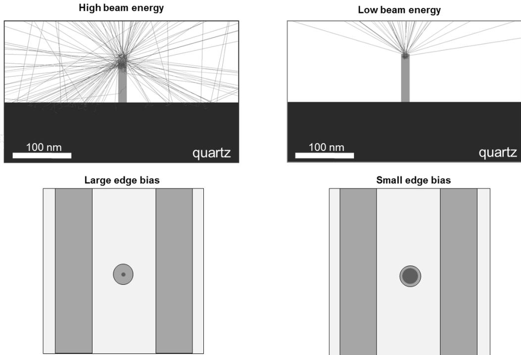
Figure 5: Upper part: Simulations of the electron trajectory for an isolated defect in cross section for a high (left side) and low beam energy (right side), respectively. Lower part: Top view of the defect with the area exposed by the electron beam in a darker shade. This demonstrates a direct relation between the beam energy and the minimum repairable feature size defined by the smaller process bias
