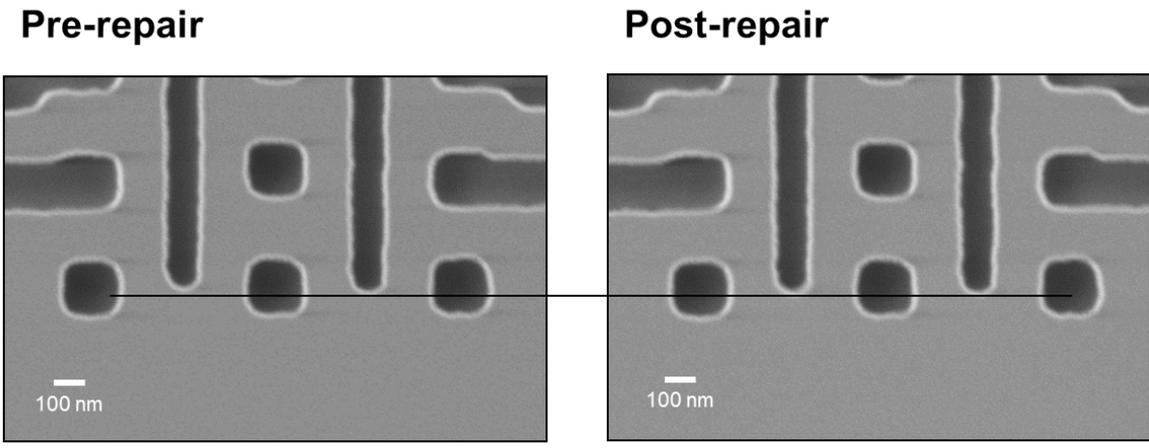
Figure 6: A 15 nm line shortening defect was successfully repaired by applying a low energy e-beam-based repair process
