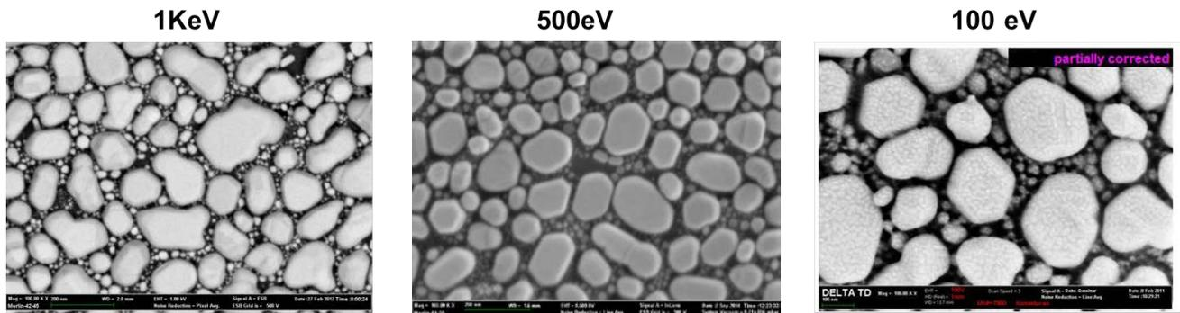
Figure 3: Representative gold on carbon resolution samples for a MERLIN e-beam column at 1000 eV (left) and 500 eV (center). An aberration corrected image taken at 100 eV using a dedicated low-voltage microscope from Carl Zeiss Microscopy is shown on the right.
