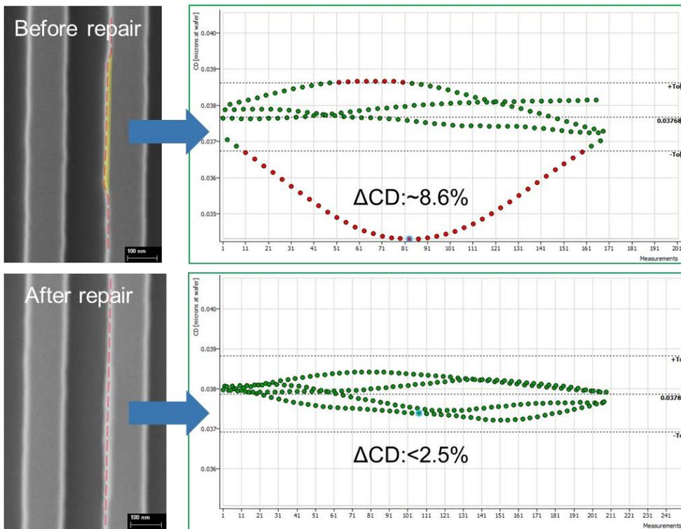
Figure 8: Example of complicated 10 nm x 500 nm defect on an A6L2 reticle. Upper left: SEM image before repair. Upper right: AIMS measurement is predicting a delta CD of -8.6 %. Lower left: Post repair SEM image. Lower right: same AIMS measurement was performed. The measured delta CD is below 2.5% which means a successful repair.
