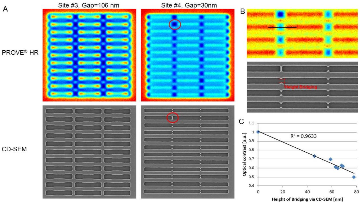
**Figure 8:** Comparison of PROVE® HR images against SEM data.
