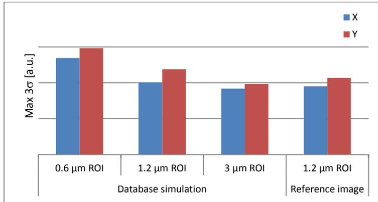
**Figure 5:** Repeatability of dense contact array for varying ROI sizes and correlation measurement methods (128 sites across the mask area, 10 loops).
