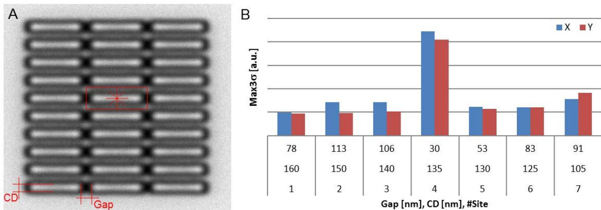
**Figure 7:** Registration repeatability performance of bar structures.
