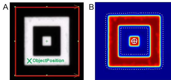
**Figure 1:** Keyhole functionality for nested objects. Per default all correlation methods take all pixels within the ROI (red rectangle) into account.
