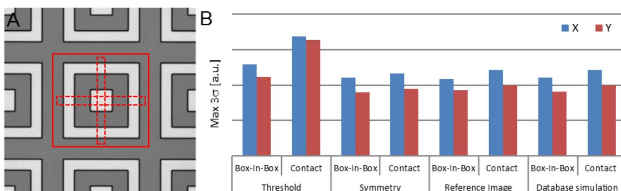
**Figure 2:** Measurement setup and repeatability performance of a standard Box-In-Box feature on a EUV mask.
