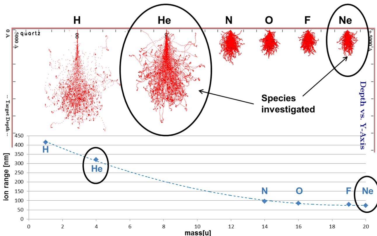
Figure 2: SRIM Monte Carlo simulation of scattering events and corresponding ion ranges for various light ions<sup>2</sup>.
