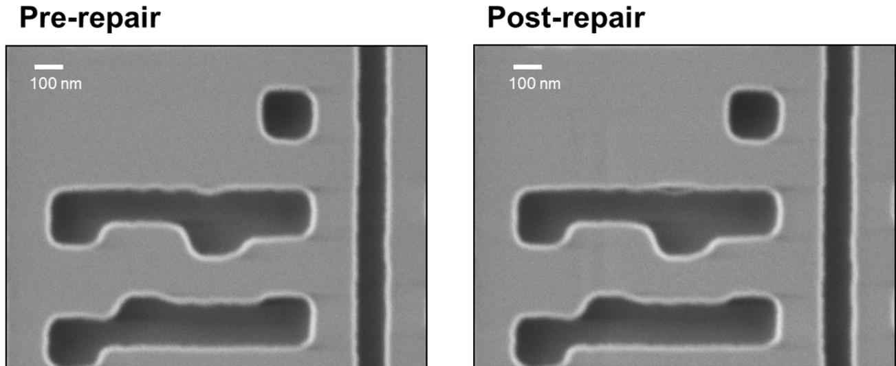
Figure 7: A 16 nm extension defect was repaired successfully by applying a low energy e-beam based repair process
