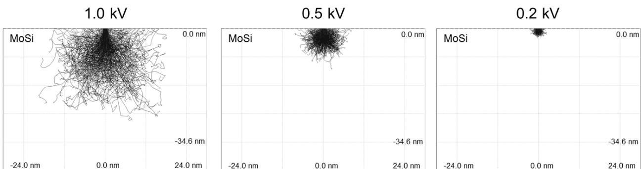
Figure 1: Comparison of electron/solid interaction volumes at different primary beam energies as simulated by Monte Carlo calculations (software: CASINO). The solid is a MoSi absorber material, while the beam radius was set to 1 nm.
