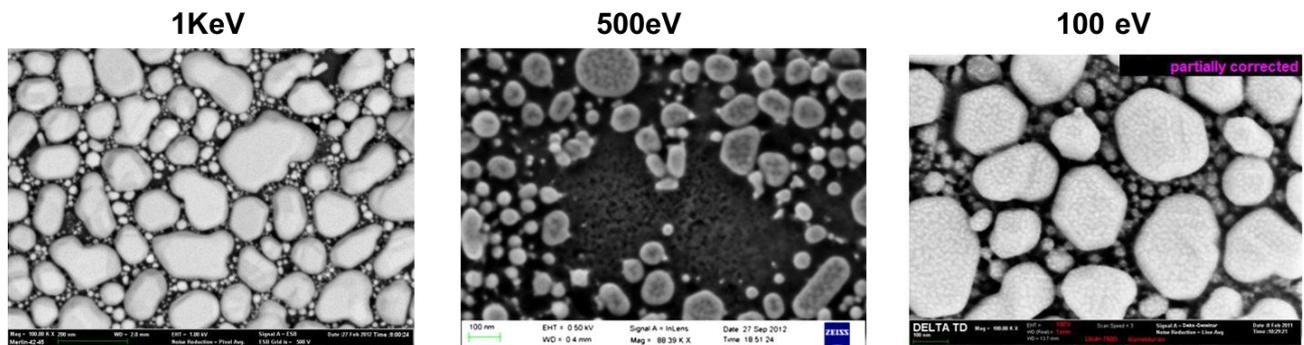
Figure 3: Representative Gold on Carbon resolution samples for a MERLIN e-beam column at 1000 eV (left) and 500 eV (center). A aberration corrected image taken at 100 eV using a dedicated low-voltage microscope from Carl Zeiss Microscopy is shown on the right.
