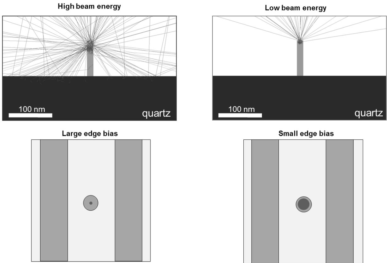
Figure 5: Upper part: Simulation of the electron trajectory for an isolated defect in cross section. The lower part shows a top view of the defect with the area exposed by the electron beam in a darker shade. This demonstrating a direct relation between the beam energy and the minimum repairable feature size defined by the smaller process bias
