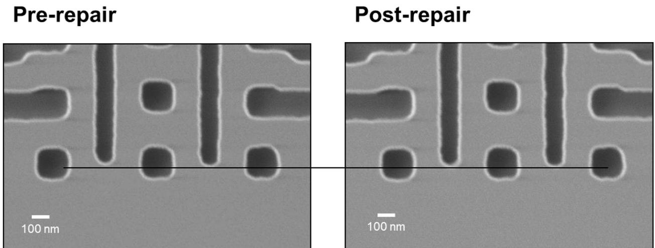
Figure 6: A 15 nm line shortening defect was repaired successful by applying a low energy e-beam based repair process
