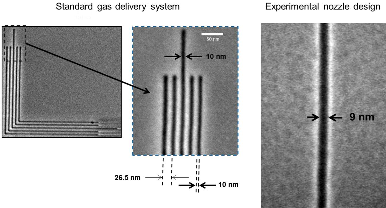
Figure 4: A dense line and space pattern was etched into quartz material by e-beam induced processing. An etching resolution of 10 nm could be achieved. For an optimized nozzle design the resolution was about 9 nm.
