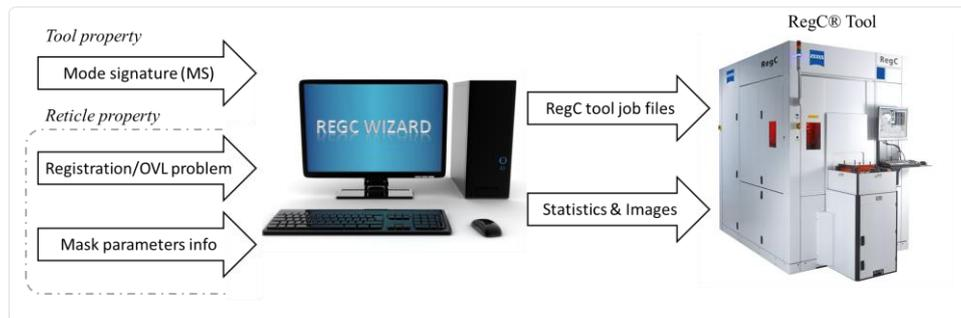
Figure 6. Inputs/outputs of the supporting software: the RegC<sup>®</sup> Wizard. The mode signature is an important input parameter to optimize the mask fingerprint.
