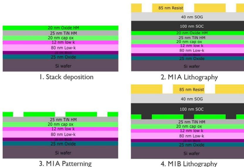
Figure 6. Schematic representation of the lithography process flow.
