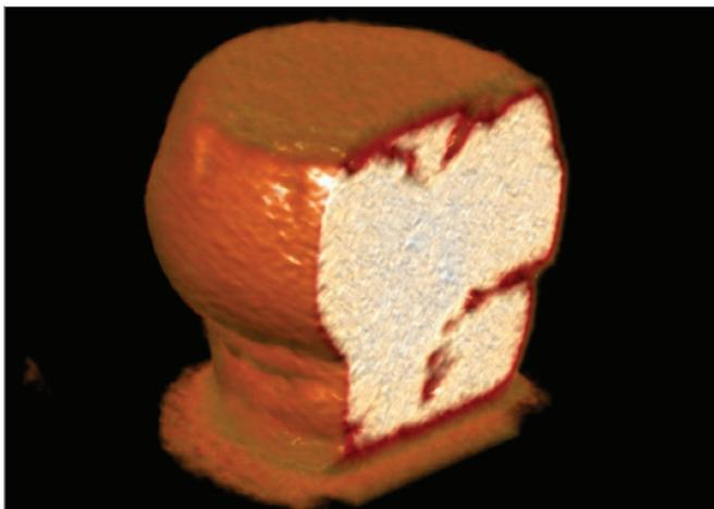
Figure 1: Cracking in solder bump (subset of image of intact package) – Xradia Versa
