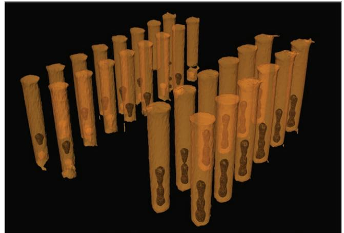
Figure 2: Voids in through silicon vias – Xradia Ultra
