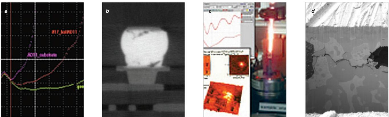
Figure 4: Images showing a new failure analysis workflow [a] Electrical testing [b] Virtual cross section using Xradia Versa [c] Progressive characterization [d] destructive cross section
