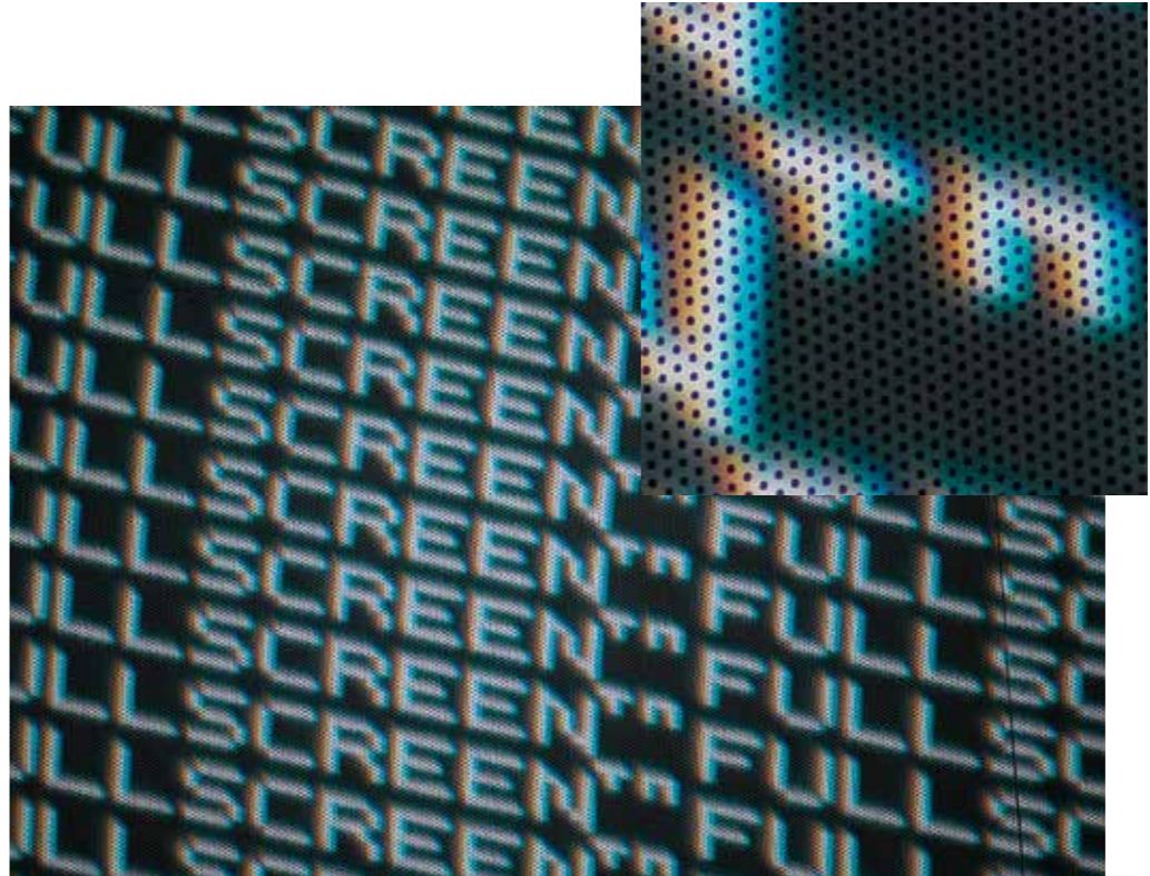
Segment of projected image, F35/NAVITAR HM117/11.7 – (test image) Lateral color: clearly visible – 2 to 3 pixel widths Exposure data: Canon EOS 5D Mk II, ZEISS Macro-Planar 2/100
